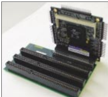
Figure 3. ISA Passive Backplane – PC/104 uses the same ISA signals found in the standard desktop PC. The one minor difference is a low 4mA current on the PC/104 data bus whereas the desktop environment specifies 20mA. The MZ104 pictured here is coupled with the Tri-M ISA10410 bus extender card allowing for quick and easy hardware prototyping with up to three ISA cards.
