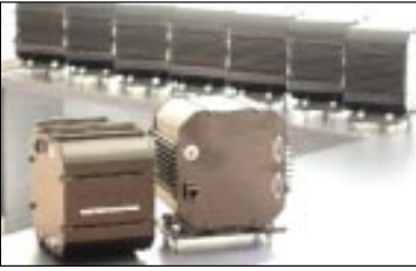
Figure 12. A typical black box solution: an embedded router — A typical black-box solution, these embedded routers are used in a mobile mining application, where available power is noisy with occasional spikes of several hundred jewels to say nothing of the constant shock and vibration the unit is subjected to day in and day out. Inside each is a PC/104 stack of cards consisting of a Tri-M vehicle DC to DC power supply, UPS battery backup, and an Ethernet card and CPU, which boots a Linux kernel and application. This is the quintessential black-box solution collecting serial data, packaging this data, and passing it along via the Ethernet port to a wireless communication system. Perhaps there is a place for white-box solutions in a black-box world.
