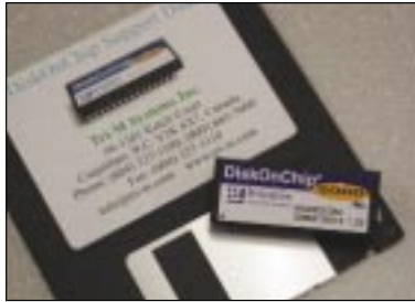
Figure 4. 64 Mbytes/sec DiskOnChip with support floppy disk – A 64 Mbytes/sec DiskOnChip and its support software. The DOC is by far the most widely supported bootable flash device on the market today with almost every manufacturer of single-board computers offering support for this family of products. Due to its ease of use, scalability, and reliability, the M-Systems product line makes an ideal digital storage device for new advanced set-top box and other embedded applications.
