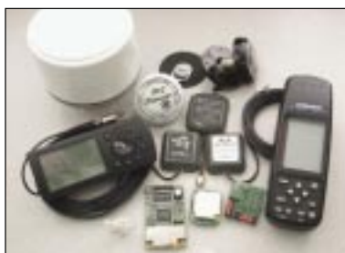
Figure 8. Current state of GPS technology – A collection of readily available commercial-off-the-shelf GPS hardware, this assortment of handheld receivers from Garmin and Loranice are shown together with a collection of Tri-M magnetic and bulkhead mounting Mighty-Mouse 1 & II and SkyMaster active antennas. Also shown are two OEM GPS receivers, an electronic compass, a DGPS, and Coast Guard data correction beacon receiver. Note: the center middle antenna was adopted by US Marine Corps Warfighting Labs, which deployed more than 900 of these units to collect tracking data on individual soldiers involved in large scale training exercises.
