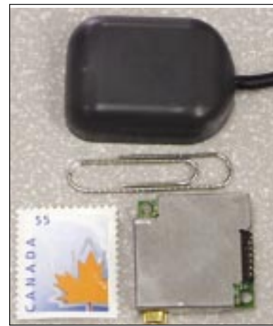
Figure 11. 2001 GPS technology soon to be released – Shortly after this article is published, Tri-M will release the REB2200 from Royaltek. This is an amazingly small, 23mm x 23mm, 3.3VDC 12-channel GPS receiver. Using the SirfStar-II chip set, it supports both DGPS and WAAS demodulation for greater output accuracy. Tri-m's Micro Sykmaster shown on top, is an active ceramic patch GPS antenna built around a 24Db gain, low-noise amplifier that consumes a mere 11mA.
