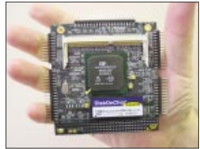
Figure 1. MZ104 board in the hand – One of the first five original beta test MZ104 boards. This unit was designed, built, and tested in less than 60 days. Shown without the SO_DIMM memory module, main memory can be added in sizes 2 to 64 Mbytes using fast SDRAM. Heat is not a problem as the MachZ chip consumes less than 0.5 Watts of saving battery power, or engineering additional heat dissipation in sealed enclosures.
