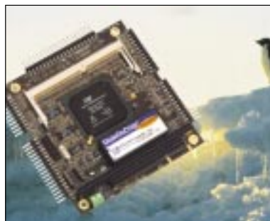
Figure 7. MZ104 with Penguin – The MZ104 is capable of booting Linux or any of a host of other operating systems. As with standard desktop hardware, the MZ104 can boot and run programs from a floppy disk, or an IDE hard disk drive, in addition to supporting a boot from DiskOnChip or easily booting your code embedded in Flash memory above and within the BIOS Flash device.
