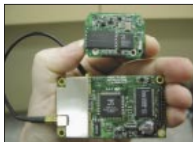
Figure 9. GPS receivers circa 1999 and 2000 – Two GPS receivers in the hand show the progress made during the last 18 months in this arena. The larger unit, an REB12R (71 x 41 x 7mm), is a 12-channel receiver, DGPS-ready, and the smaller unit is an REB2100 (40 x 31.5 x 6.5 mm) DGPS- and WAAS-ready receiver and weighs a minuscule 8.6 grams. Both receivers will reacquire satellite signal lost due to the effects of urban canyon or foliage environments in an incredible 0.1-second. Both of these OEM receivers are priced below 100.00 USD in small quantities.
